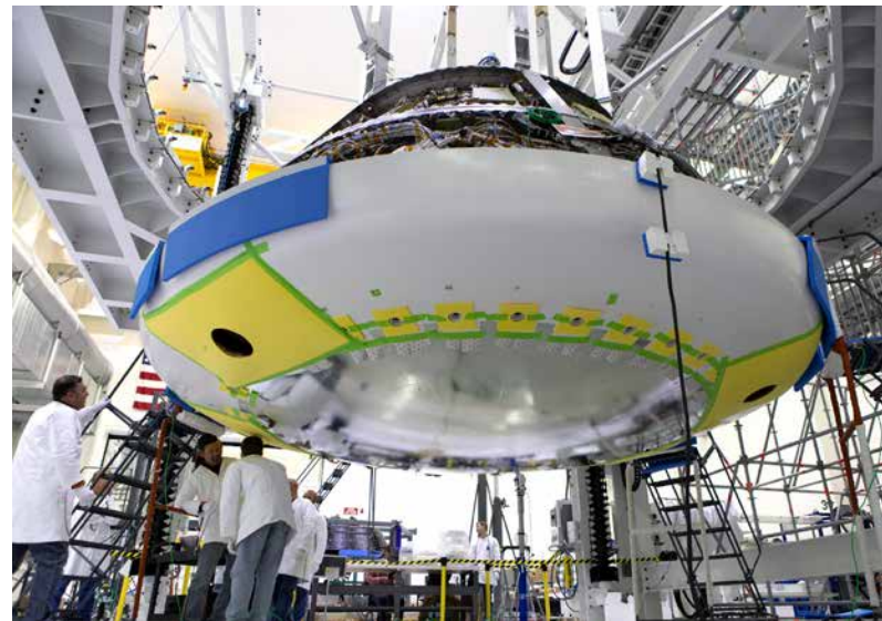
Above: Engineers and technicians check fittings during installation of the heat shield to the Orion crew module July 25, 2018, at NASA's Kennedy Space Center. Image credit: NASA/Kim Shiflett
