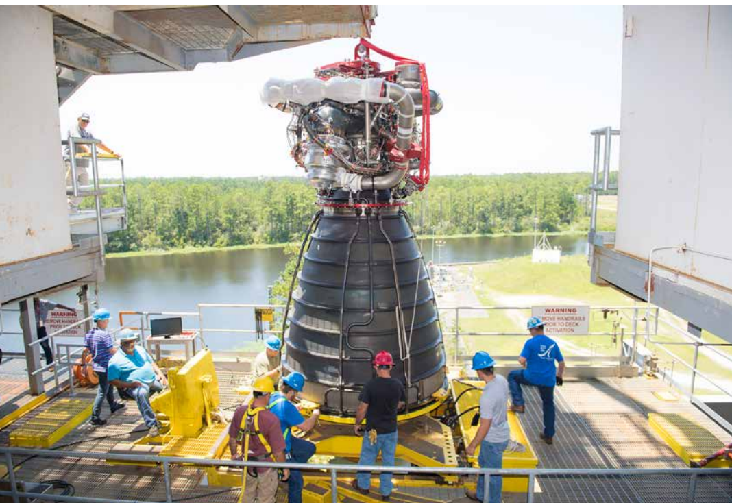
Left: A team prepares an RS-25 engine No. 0525 for installation on the A-1 Test Stand at Stennis Space Center on July 23, 2018, in preparation for SLS hotfire tests. Four RS-25 engines, working in conjunction with a pair of solid rocket boosters, will help power the SLS rocket at launch. Image credit: NASA
