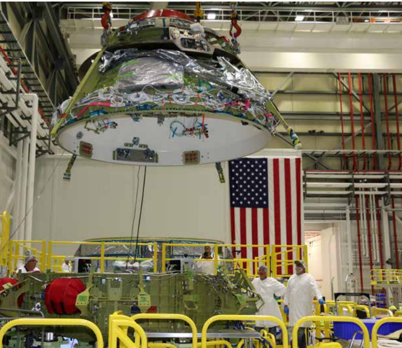
Above: The upper and lower domes of the Boeing CST-100 Starliner Spacecraft 2 Crew Flight Test Vehicle were mated June 19, 2018, inside the Commercial Crew and Cargo Processing Facility (C3PF) at Kennedy Space Center in Florida. The Starliner will launch astronauts on a United Launch Alliance Atlas V rocket to the International Space Station enabled by NASA's Commercial Crew Program. Image credit: Boeing
