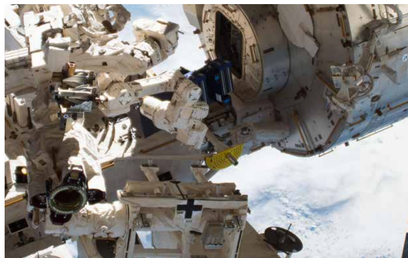
Above: The blue MISSE-FF and the Japanese Experiment Module (JEM) Exposed Facility exit the ISS through the JEM airlock. The experiment is comprised of a structural platform that holds multiple MISSE sample carriers. Image credit: NASA
