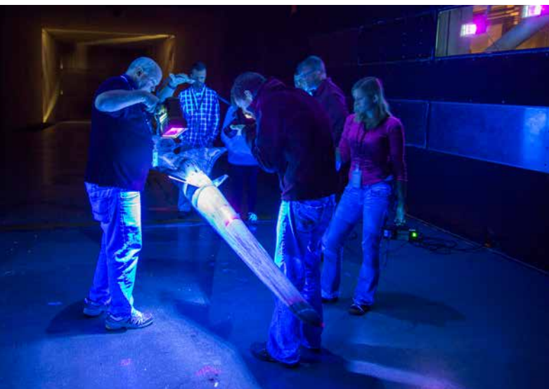
Above: Technicians examine streaks made by oil along the body of a model of the QueSST X-plane after a test in the 14 x 22 wind tunnel at Langley Research Center. The oil, which was released into the wind tunnel's airstream, shows how the air moved around the shape of this design for a quieter supersonic aircraft. Image credit: NASA
