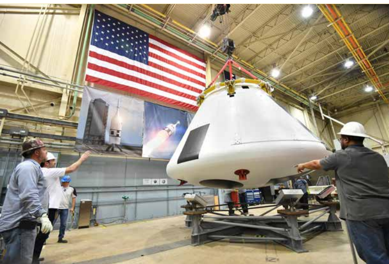
Above: Technicians lower the crew module for Ascent Abort-2 onto a stand at the Johnson Space Center on March 2, 2018. Image credit: NASA/Robert Markowitz
