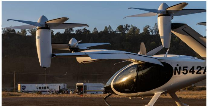
Joby's all-electric vertical takeoff and landing (eVTOL) aircraft is pictured at the company's Electric Flight Base, located near Big Sur, California. NASA began flight testing with the aircraft as part of the Agency's Advanced Air Mobility (AAM) National Campaign. This test runs through September 10, 2021. Image Credit: Joby Aviation
