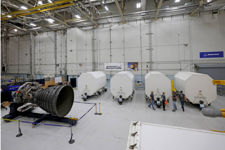
Four Artemis II engines in their shipping containers and the RS-25 “pathfinder” engine
