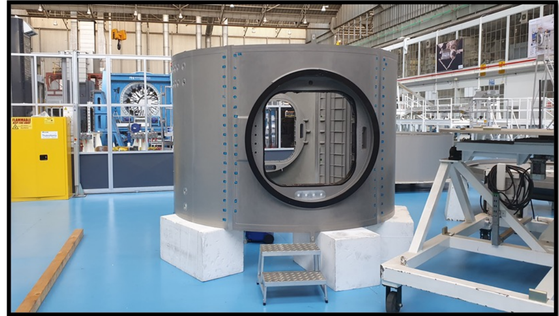
HALO Habitable Element (HE) Longitudinal Welds Completed
