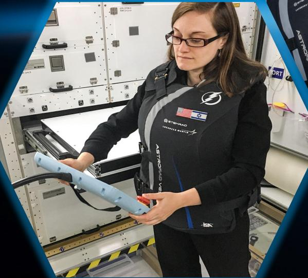
*Top left: The AstroRad Vest undergoes fit testing at the Kennedy Space Center in the Lockheed Martin mockup of the Gateway*
