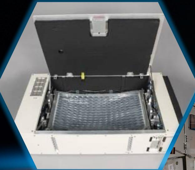
*Top Left: Brine Processor's dual membrane bladder works to recover additional water from urine brine.
