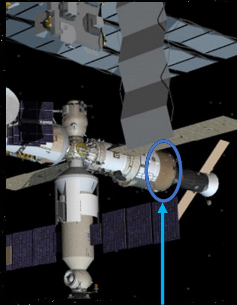
ISS Atmosphere Leak Location
