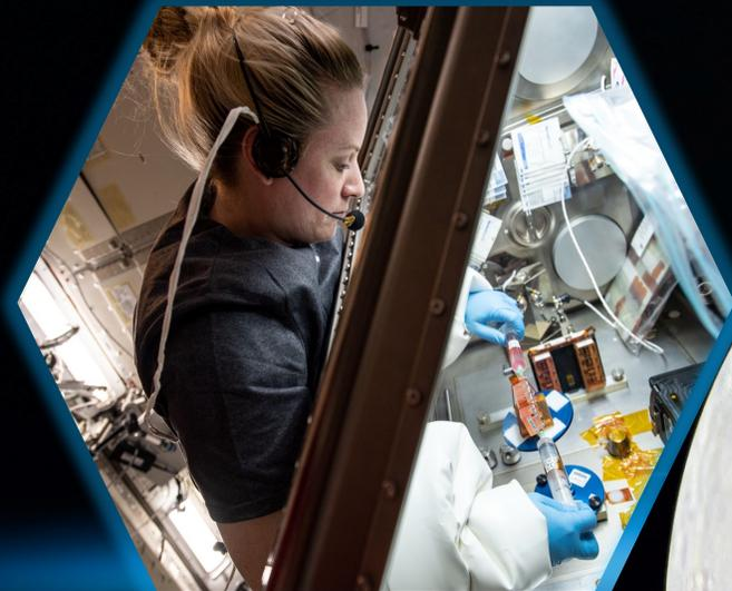
Top Left: NASA astronaut Kate Rubins works inside the Life Sciences Glovebox (LSG) to change the Media in a Tissue Chamber for the Cardinal Heart experiment.
