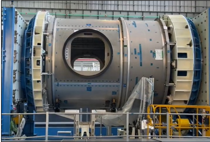
HALO structure in the friction stir weld machine (TASI, Italy)
