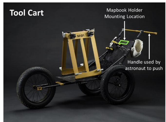
Figure 1: Tool Cart showing approximate mapbook holder mounting location.
