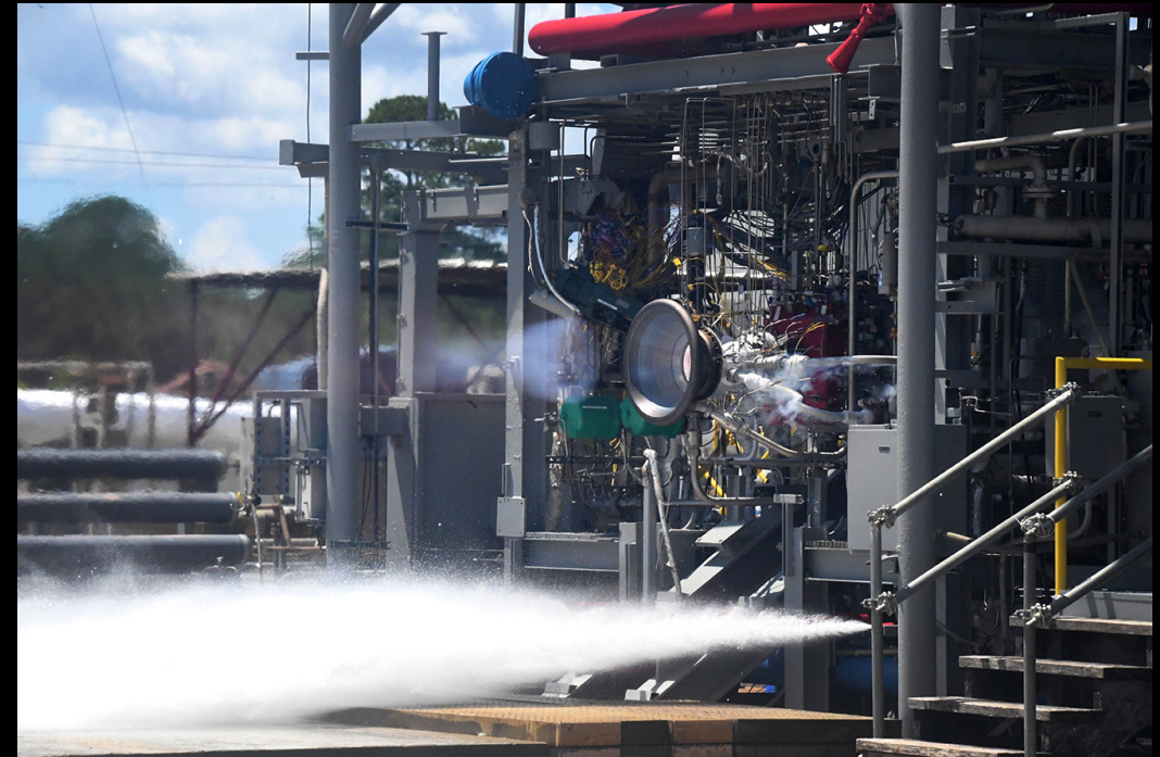
Lemnings (LEO Mid-scale channel wall nozzle) for SLS – testing at MSFC Test Stand 116
