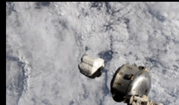
Supporting commercial growth in LEO with 24 Commercial Facilities on-orbit: Nanorack airlock deploying trash on ISS
