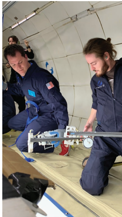
A spacecraft boom is deployed during a parabolic flight. Credit: North Carolina State University
