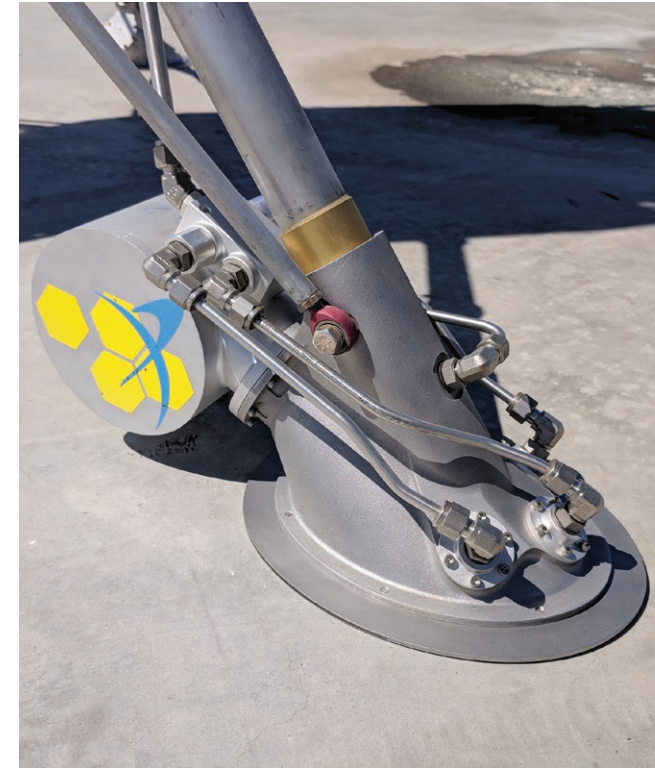
Successful Flight Opportunities–supported tests of PlanetVac, which is designed to attach to the leg of a lander vehicle (as shown here), helped the technology be selected for Artemis as part of a CLPS mission. Credit: Honeybee Robotics
