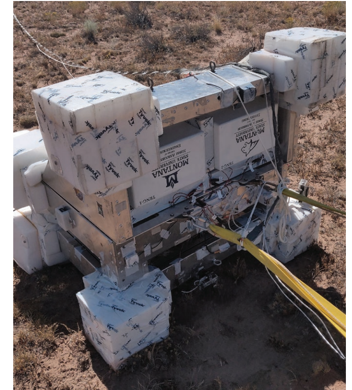
Flights facilitated by Flight Opportunities, including on high-altitude balloons and rockets, helped mature the RadSat technology (shown at the recovery stage after a World View Enterprises balloon flight) for Artemis selection. Credit: World View Enterprises
