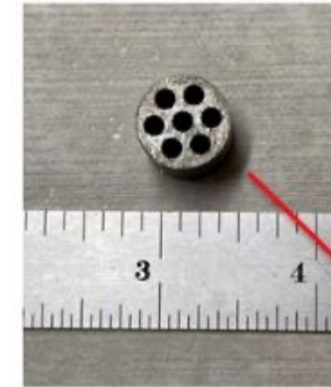
CERCER fuel compact for Sirius-2C experiment
