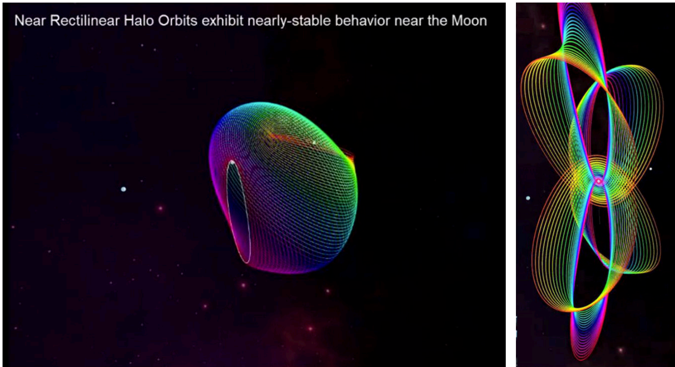
Figure 2. Illustration of the family of NRHOs; the Artemis – Gateway selected NRHO is highlighted in white on the left image.
