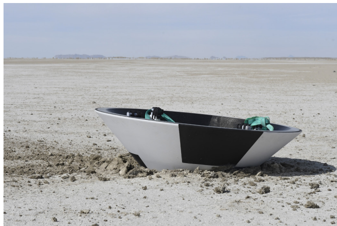
NASA is conducting drop tests at UTTR using realistic prototypes of the MSR EES at speeds comparable to what would occur during an actual landing event. Photo credit: U.S. Air Force/NASA
