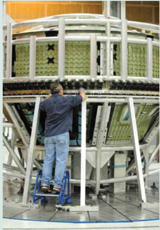
(Right) On May 27, 2010, a weld technician looks on as the bulkhead and nosecone of the Orion spacecraft are joined using friction stir welding at NASA's Michoud Assembly Facility in New Orleans. The vehicle was inverted in the tool for this weld.
