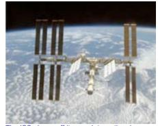
The ISS shows off its new International Partners elements—the European Space Agency's Columbus module, Japan's Kibo Pressurized Module and Logistics Module (all three located where the main body of the ISS meets the truss in the photo), and Canada's Dextre robotic arm—as Space Shuttle Discovery pulls away at the end of STS-124 in June 2008. (Credit: NASA)
