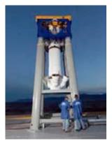
Technicians at Alliant Techsystems (ATK) in Utah inspect the facility's new test stand, which contains the inverted, full-scale inert abort motor for the Orion crew capsule's launch abort system. The abort motor, which anchors atop the capsule, is designed to pull Orion and its crew safely away from the Ares I rocket in the event of a mishap on the launch pad or during the first 300,000 feet of the launch. (Credit: ATK)
