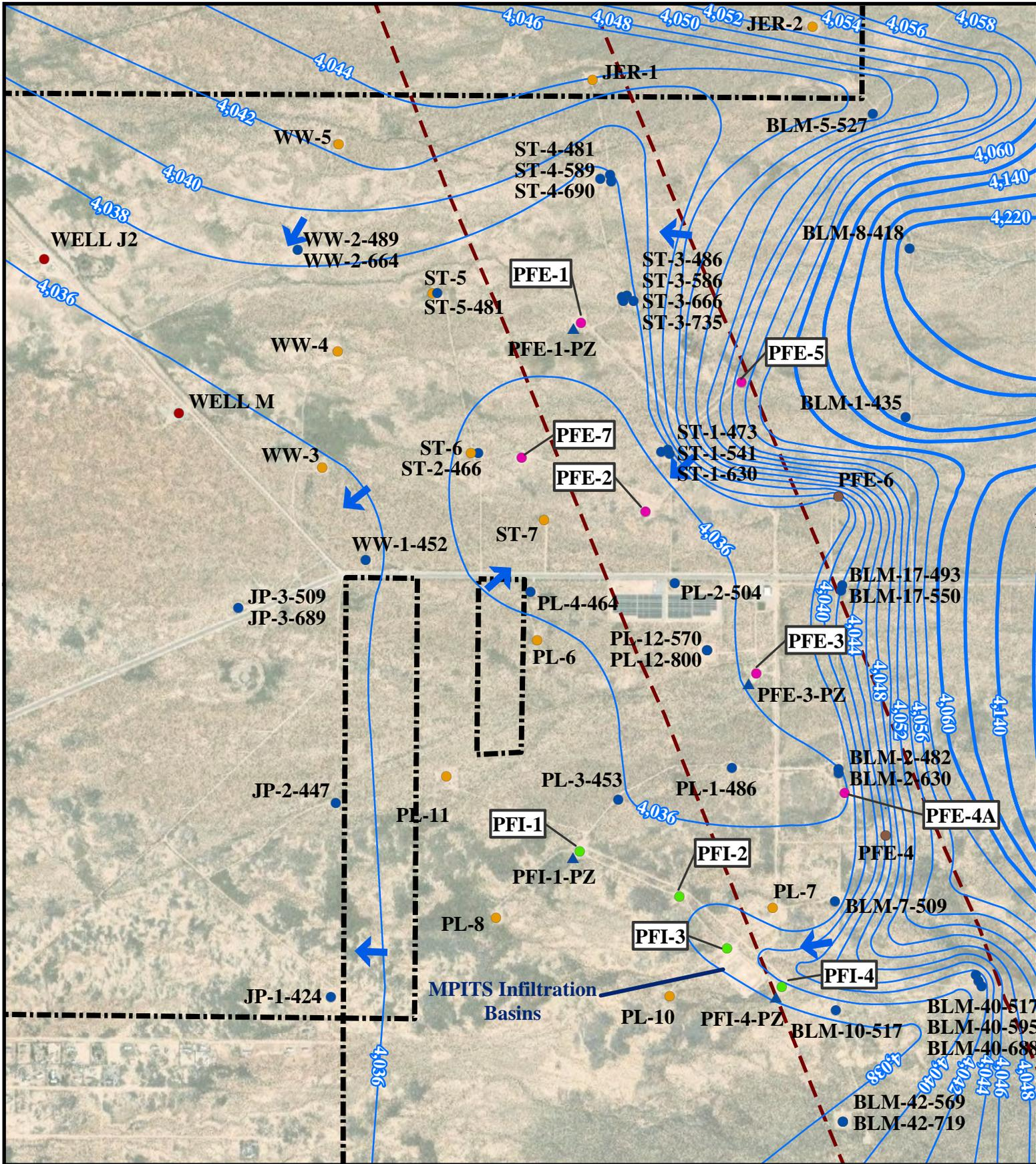
**Plume Front Groundwater Elevations for First Quarter 2023**
