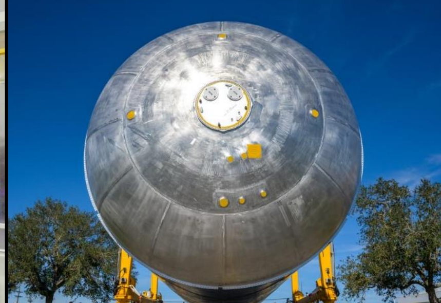
ARTEMIS III CORE STAGE LH2 TANK
