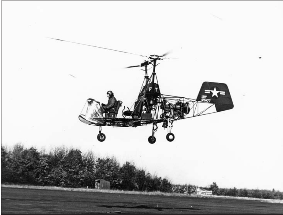
FIGURE 5.34. Kaman combined a Boeing 502 gas turbine engine with his synchropter rotors and servo-flap cyclic control system to create the pioneering K-225 in 1951. (NASM, Smithsonian Institution [SI 2002-958])
