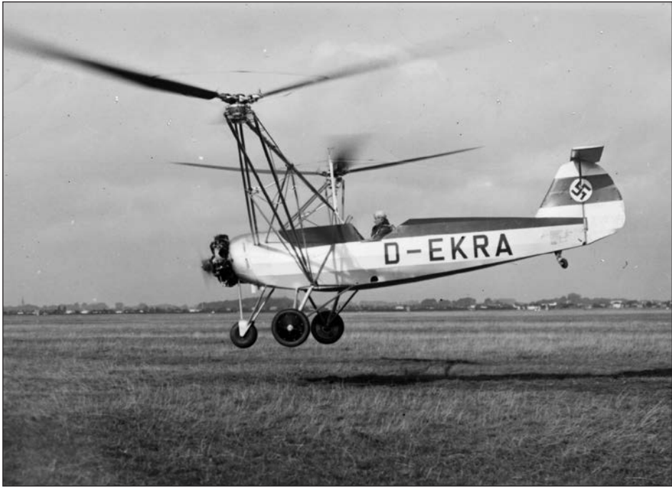
FIGURE 5.28. The twin-rotor Focke-Achgelis FA-61 was the first fully controllable helicopter when it flew in June 1936. (NASM, Smithsonian Institution [NASM A-2316])
