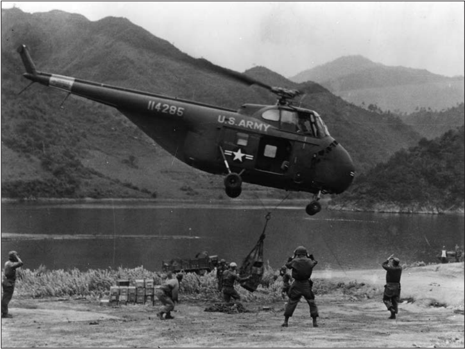
FIGURE 5.40. Although the aerial evacuation of wounded soldiers is the persistent image of the helicopter's role in Korea, combat helicopters, primarily the Sikorsky H-19C Chickasaw, also delivered supplies and other valuable cargo to soldiers in the field. (United Technologies Corporation Archive via NASM, Smithsonian Institution [NASM 00088684])
