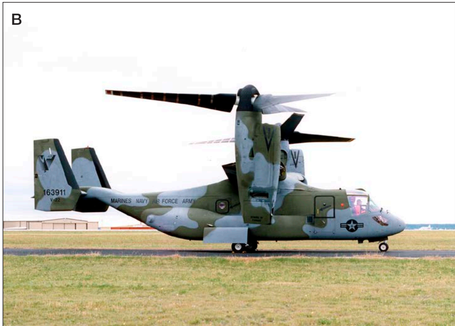
FIGURE 5.39. (A) The Bell XV-15 is shown in forward flight. (Courtesy of Bell Helicopter Textron, NASM, Smithsonian Institution [SI 92-15093]) (B) The technical offspring of the XV-15, the Bell-Boeing V-22 Osprey, is shown in its vertical takeoff orientation. (NASM, Smithsonian Institution [97-15252])
