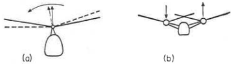
FIG. 2-8. Methods for obtaining lateral control. (A) Tilt of rotor thrust (B) Differential thrust change.
