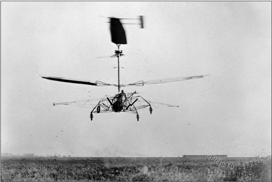
FIGURE 5.21. The Italian Corradino d'Ascanio reached an altitude of 60 feet in his coaxial helicopter in 1928 and proved to a skeptical public that helicopters could fly higher than a few feet. (American Helicopter Society Copy Negative Collection, NASM, Smithsonian Institution [NASM 9A00958])
