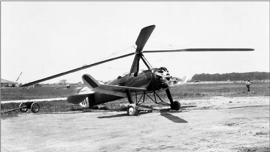
FIGURE 5.26. The NACA conducted an investigation of an experimental cantilevered, three-bladed rotor on the Pitcairn PAA-1 autogiro beginning in 1933. (NASA Image # L-05662 [Langley Research Center, or LaRC])
