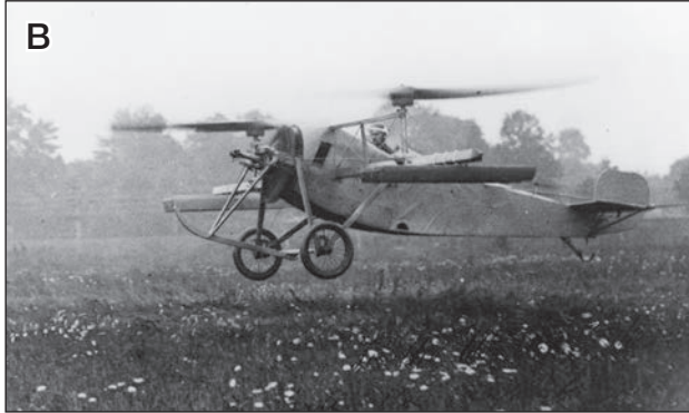
FIGURE 5.20. (A) The twin “rotors” on Paul Cornu’s 1907 helicopter were paddles attached to horizontal bicycle wheels driven by a 24-horsepower engine. (American Helicopter Society Copy Negative Collection, NASM, Smithsonian Institution [NASM 9A00883]) (B) The Berliner 1922 helicopter, seen here hovering briefly at College Park, Maryland, utilized rotors that were essentially wooden propellers with special airfoil profiles and pitch distributions. There was also a small, vertically thrusting auxiliary rotor on the rear of the fuselage. Tilting of the rotor shafts provided directional control, and a small grouping of wings in the rotor slipstream allowed lateral control. All Berliner helicopters used a conventional elevator and rudder assembly at the tail. (NASM, Smithsonian Institution [SI 77-6903]) (C) Jens Ellehammer is a national hero in Denmark for his early flight experiments. His coaxial rotor helicopter never made a free and controlled flight. (NASM, Smithsonian Institution [SI 85-3344]) (D) The Engineering Division’s quadrotor helicopter designed by George de Bothezat lifts off at McCook Field in 1922. (NASM, Smithsonian Institution [SI 77-6876])
