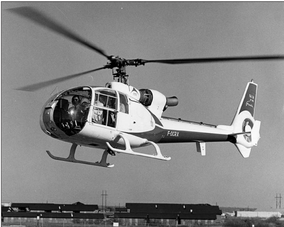
FIGURE 5.35. Aerospatiale introduced the SA.341 Gazelle in 1971 as a replacement for the highly successful Alouette II. It featured a Fenestron shrouded tail rotor and high tail fin that increased high-speed performance and protected the rotor from damage. The French and British military and numerous international operators used the Gazelle around the world. (NASM, Smithsonian Institution [NASM 7A00452])
