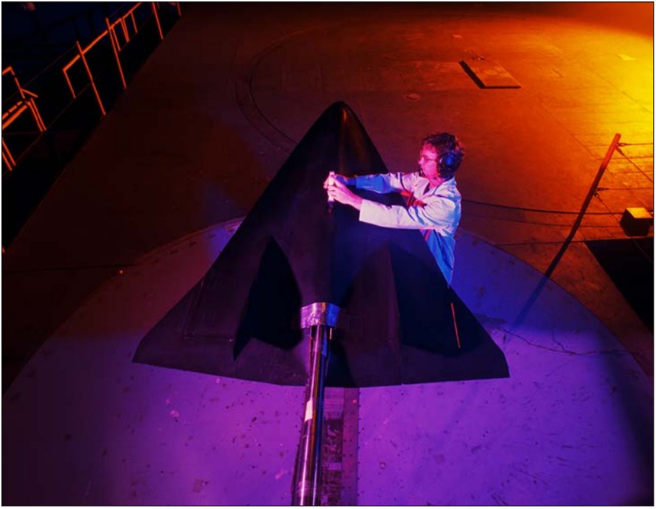
FIGURE 5.1. Pictured is Küchemann's dream of the future: a Mach 5.5 Wave Rider model in the Full Scale Wind Tunnel at Langley Research Center in the 1990s. (NASA Image #L-1995-04049 [LaRC])
