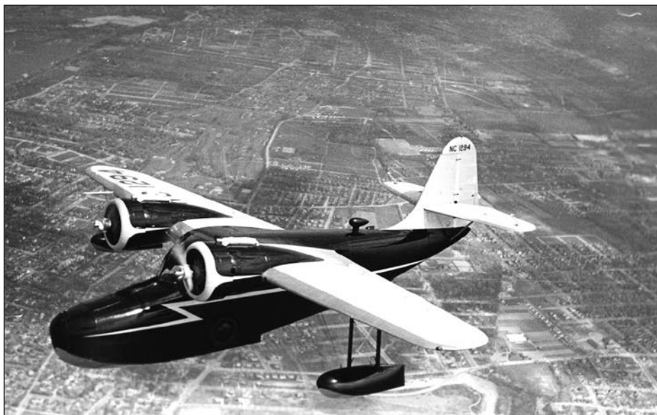
FIGURE 5.17. Amphibians such as this Grumman G-21A Goose persisted into the post–World War II era due to their flexibility in operations, especially for charter companies taking customers to exotic and hard-to-reach locales. In the 21st century, aeronautical companies have resumed production of amphibians and floatplanes due to their high demand. (Hans Groenhoff Collection [HGD-157-18], NASM, Smithsonian Institution)
