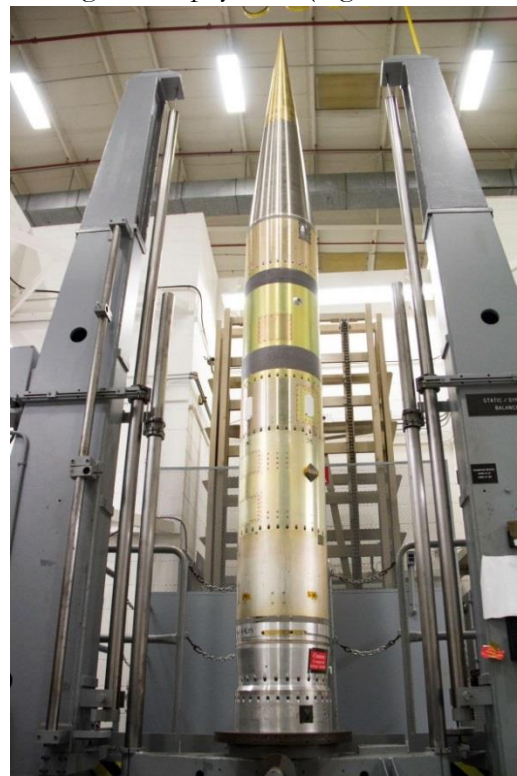
Figure 6.2.2-1 Gisholt Rocket Balancing Machine at WFF
