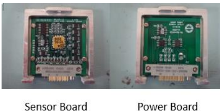
Figure 5.3.6-1: Wallops Accelerometer & Attitude Sensor Package (WAASP)
