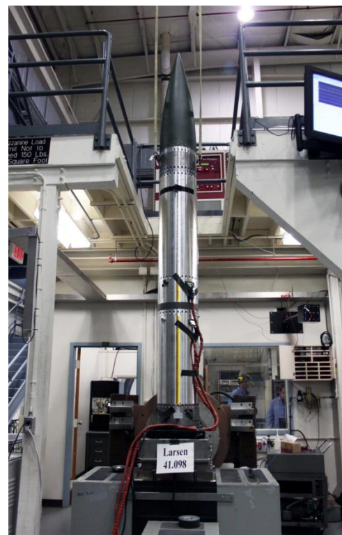
Figure 6.2.3-1: Ling Electronics B335 Thrust Axis Shaker at WFF
