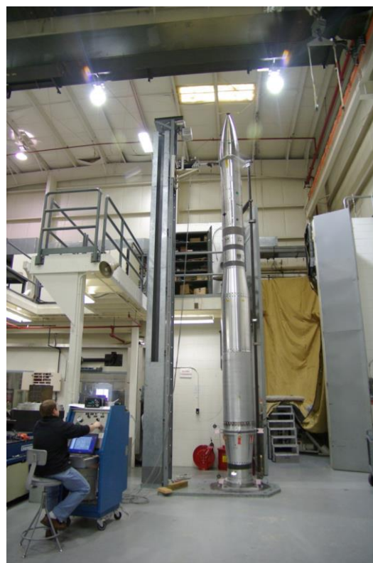
Figure 6.2.5-1: Bend Test Fixture at WFF
