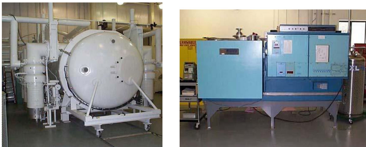
Figure 6.2.4-1 PV/T Vacuum Chamber (left) and Tenney Space Simulation System Thermal Vacuum Chamber at WFF
