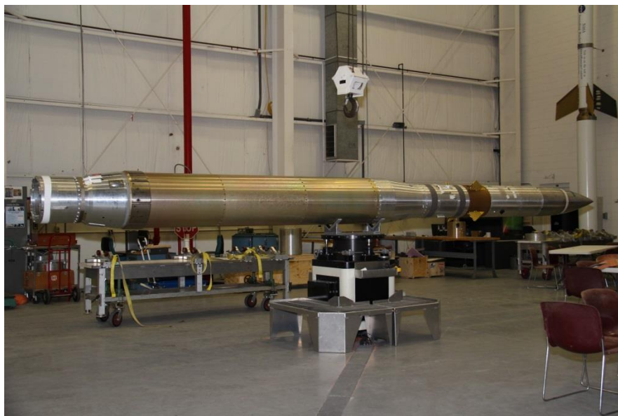
Figure 6.2.1-1 Airdyne Mark 8 Mass Properties Measurement System at WFF
