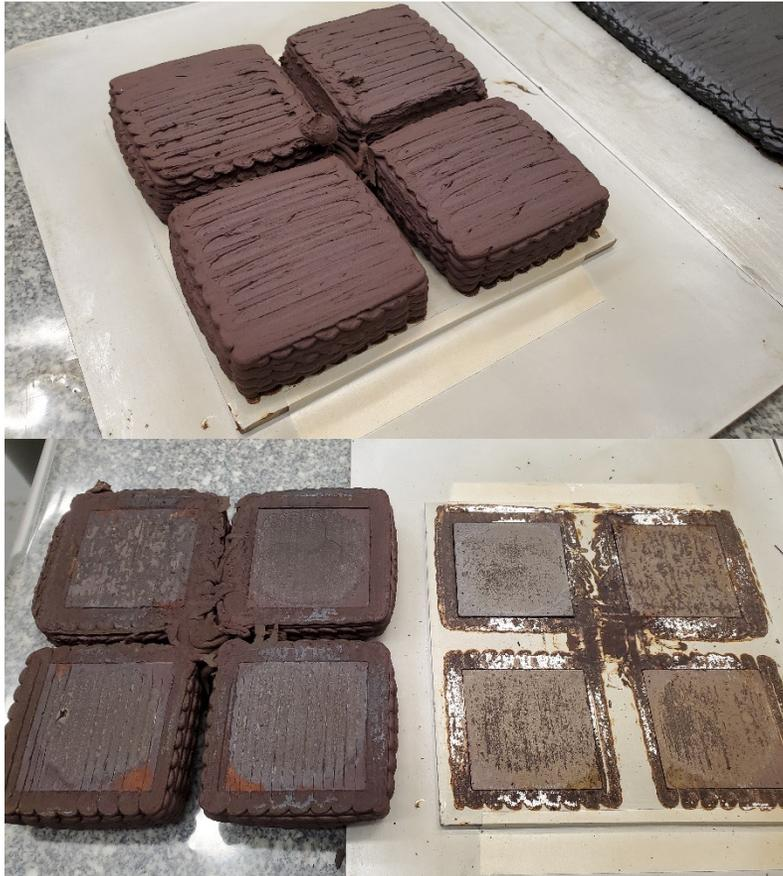
*3D printed ablative material does not stick to aluminum or titanium*
