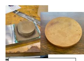
Thermal conductivity test articles
