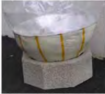
Foam stabilized antenna
