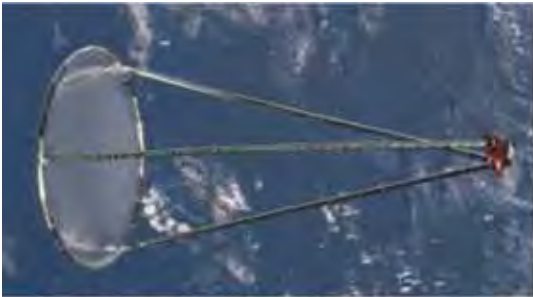
14-m-diam. inflatable antenna experiment
