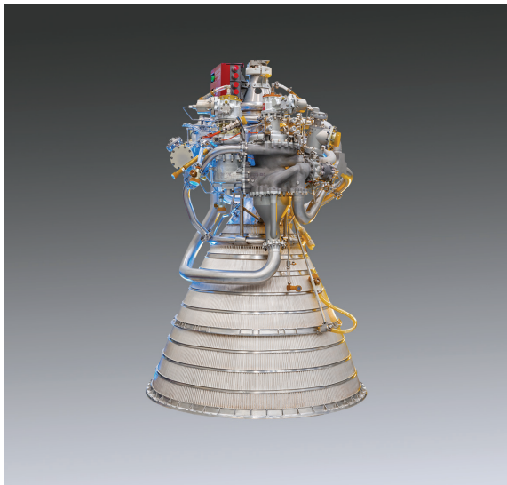
A single RL10 engine will provide nearly 25,000 pounds of thrust and serve as the main propulsion for the ICPS that will fly atop the SLS rocket Block 1 in support of each of the first three Artemis missions.
