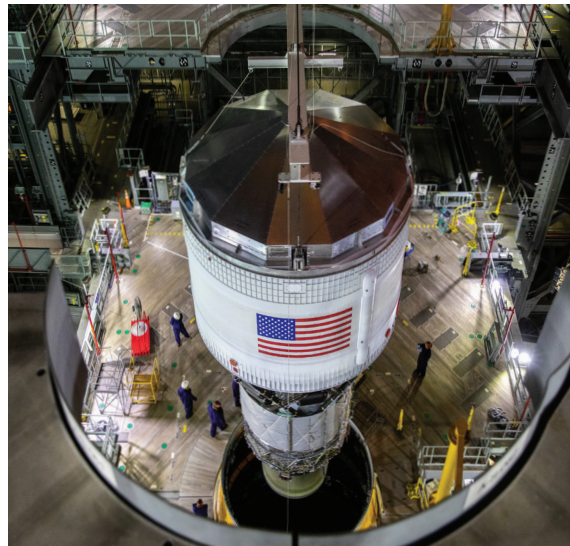
The Space Launch System ICPS mates with the launch vehicle stage adapter atop the SLS core stage in the Vehicle Assembly Building at NASA's Kennedy Space Center in Florida. The ICPS will fire its RL10 engine to send the Orion spacecraft to the Moon.
