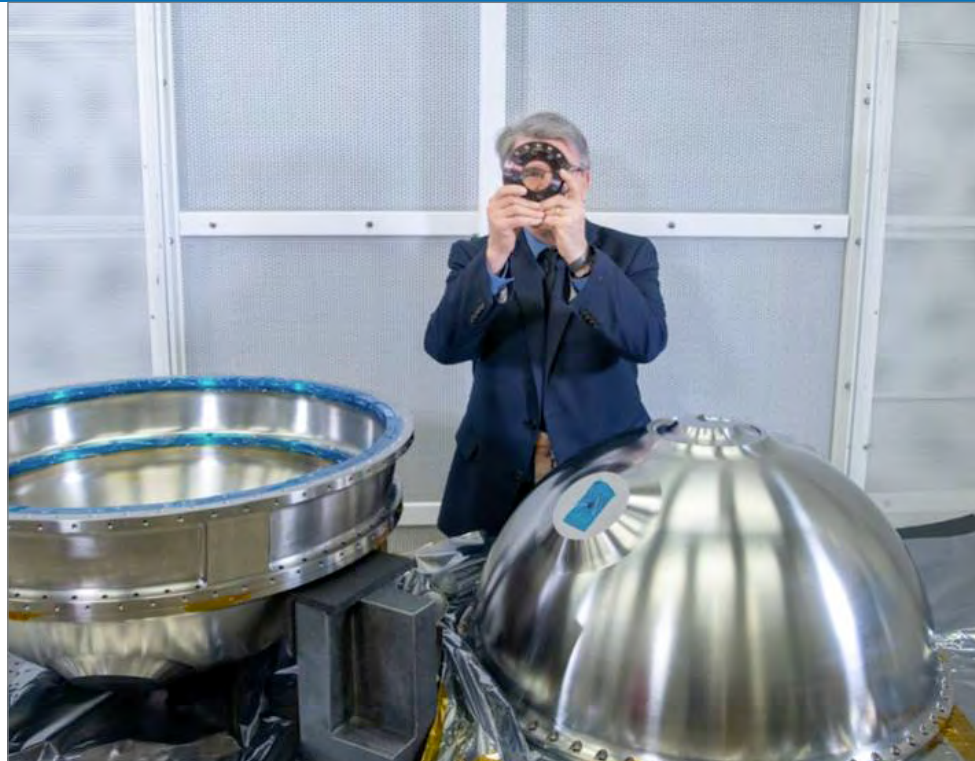
↑ Jim Garvin poses with the DAVINCI descent sphere (“probe”) engineering test unit and “the eye of Venus” (Sapphire window held in his hands). (Image credit: NASA/Goddard Space Flight Center)
