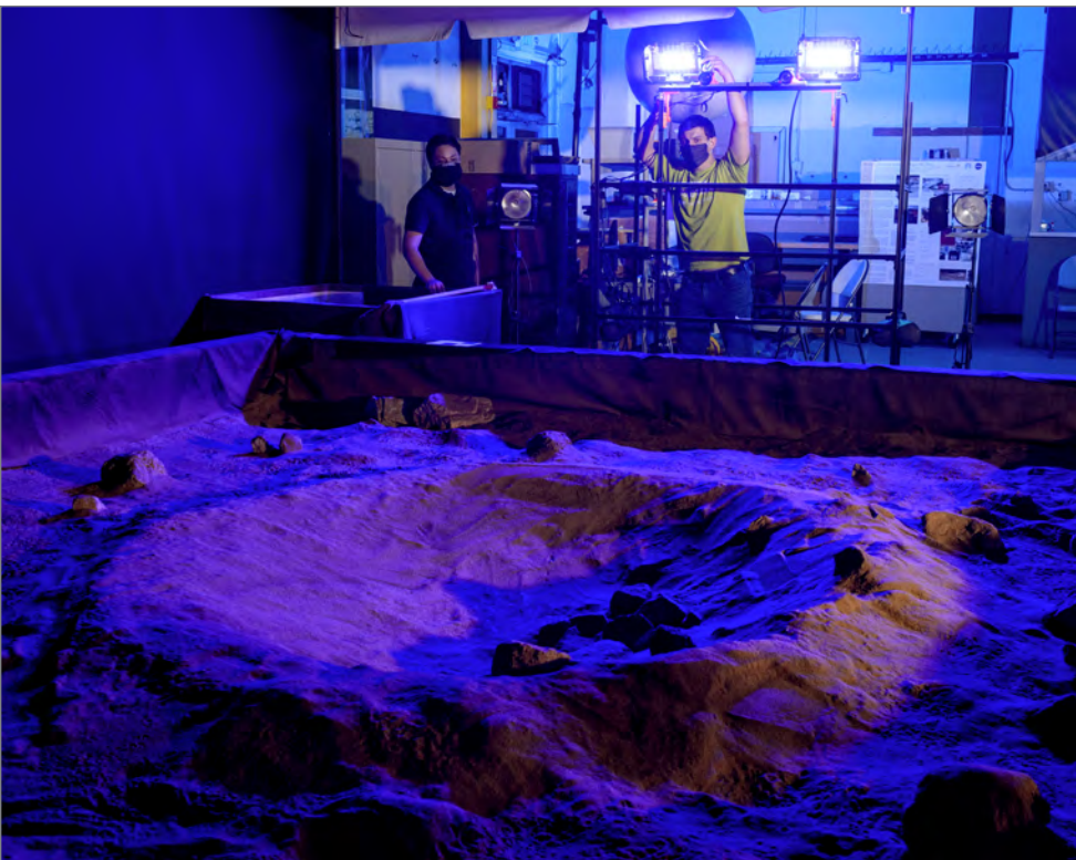
↑ At NASA's Ames Research Center, a lab designed to mimic lunar terrain as it would appear in different areas at the Moon's poles is where the VIPER team tests out lighting systems for the rover with a very low-angle illumination simulating the Sun. The VIPER team has tested several robust light-emitting diode (LED) lighting systems—including blue lights and other wavelengths—to see which would offer the best optical performance for the rover on the Moon. The Ames-based team will pass their findings on to VIPER teammates at NASA's Johnson Space Center in Houston, where the lights will eventually be built. (Image credit: NASA/Dominic Hart)
