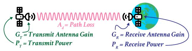
To perform a link budget calculation, we use units of decibels (dB), which express common numbers in exponential form. This is useful for expressing very large or very small numbers. To convert watts ( $P_W$ ) to decibel-watts ( $P_{dBW}$ ), use a logarithm, like so:
