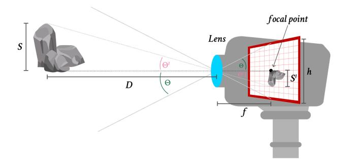
We know the focal length of the rover's camera is .5 m. Based on observations from previous missions, we know the boulder is 10 m tall. The boulder appears to be .01 m in the sensor array. Each pixel is 1x10-5 m tall.
