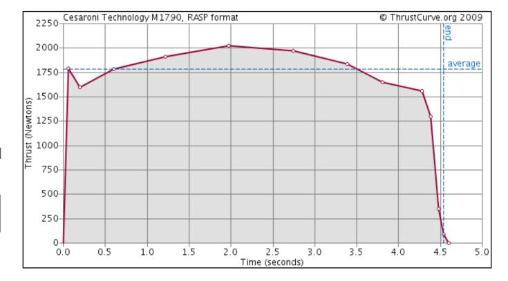
Thrust curves can be downloaded from Thrustcurve.org and imported into RockSim or Open Rocket. Practical Example of Impulse
