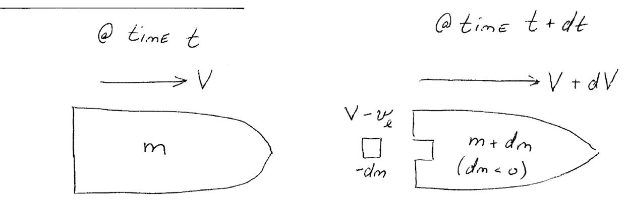
$m^*v = -(dm)(v-v_e) + (m+dm)(v+dv)$  or  $m^*v = -v^*dm + dm^*v_e + m^*v + m^*dv + dm^*v + dm^*dv$
