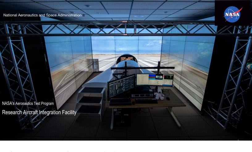
NASA Armstrong's Research Aircraft Integration Facility (RAIF) provides the ability to seamlessly integrate simulation and vehicle software and hardware systems under a single roof. This one-of-a-kind facility can simultaneously support a wide variety of advanced, highly integrated aerospace vehicles through all phases of a research program from conceptual design to flight.
