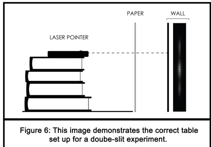
Figure 6: This image demonstrates the correct table set up for a double-slit experiment.
