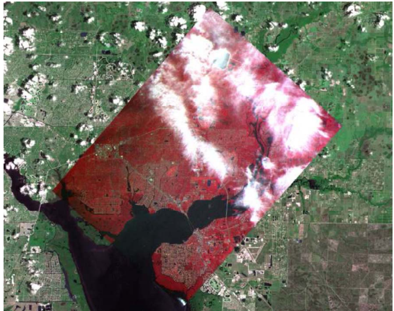
ISSAC “first light” image of Charlotte Harbor, Fla. acquired June 10, 2011, overlaid on Landsat 5 base image. The ISSAC scene is processed to highlight vegetation in red, urban areas in gray, and water surfaces in black. Clouds appear bright white.
