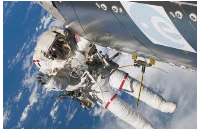
Astronaut Randolph Bresnik seen during Atlantis EVA-2 on November 21, 2009, with the unfurled AIS antenna, attached to Columbus for use in experimental tracking of VHF signals of ships at sea. (Credits: NASA)
