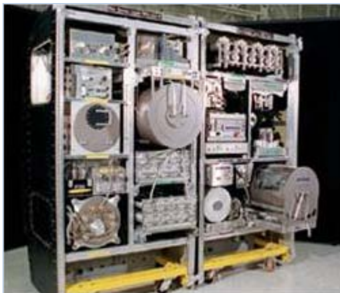
Water recycling system used on the International Space Station. Image credit: NASA/Dimitri Gerondidakis
