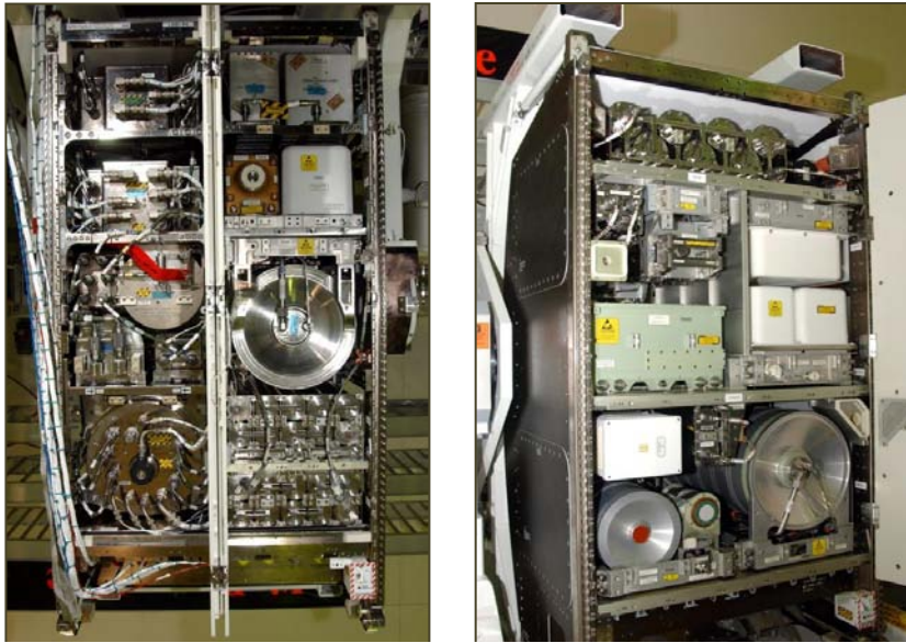
The International Space Station water recovery component of the Environmental Control and Life Support System (NASA image)
