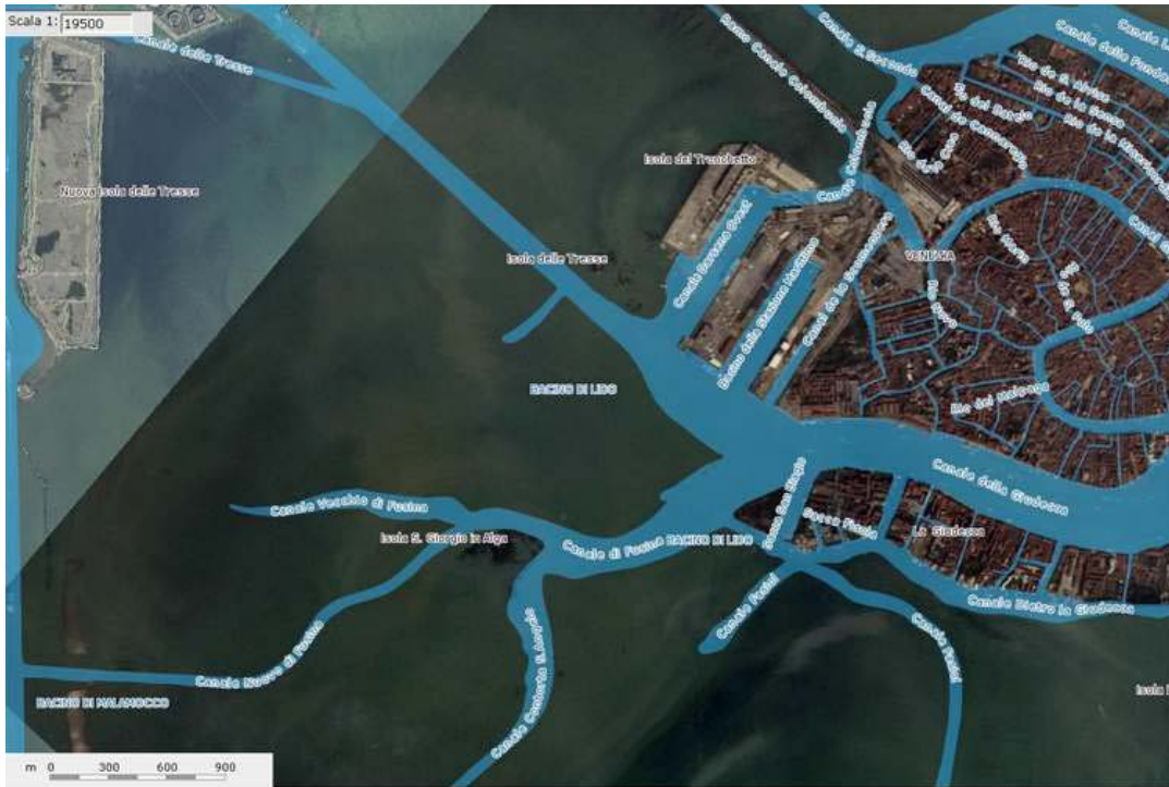
Screen capture of the Atlas of the Lagoon, showing geo-referenced astronaut photograph ISS023-E-13766 with a portion of the canal system (bright blue) added as an additional layer. The base image is an orthophoto mosaic (image created from a series of geometrically corrected images). Note that the site is currently only available in Italian. ( http://www.silvenezia.it/webgis/map.phtml?config=baseorto )
