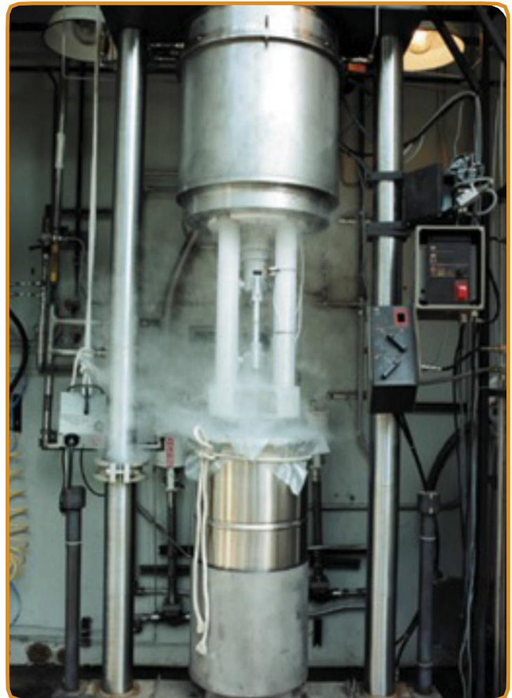
Tension Test Specimen in Liquid Hydrogen
