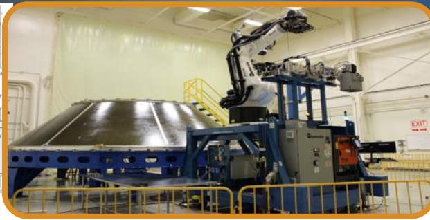
Robotic Non-Destructive Evaluation Tool
