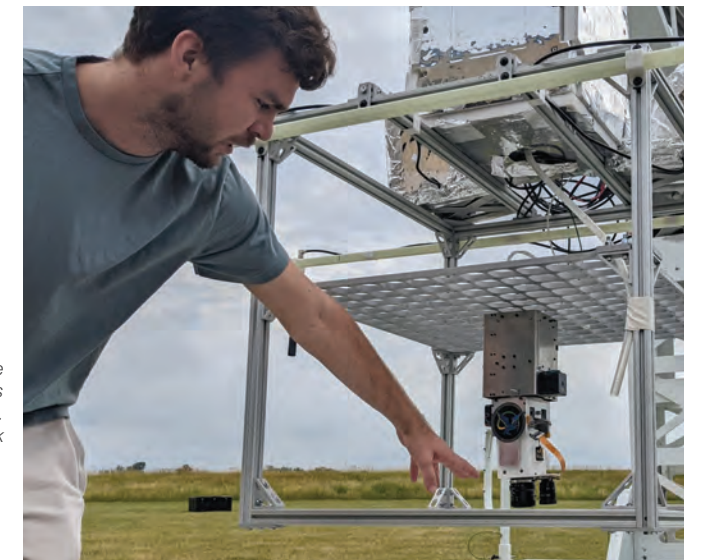
Zachary Gaines, a senior in Cal Poly Pomona’s Bronco Space Lab, points out the camera and sensor used in the team’s Bronco Ember technology to detect and track wildfires. Credits: Aerostar/Anastasia Quanbeck
