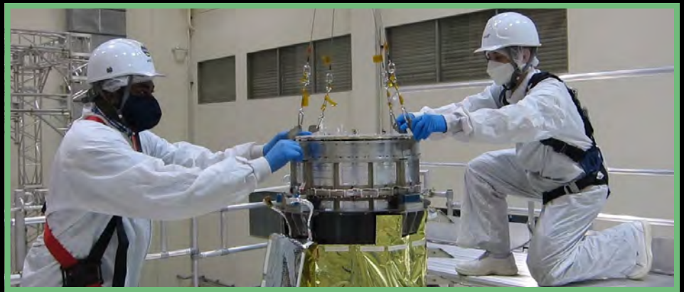
Lift and integration of the Resolve X-ray Mirror Assembly onto the top of the XRISM spacecraft at the Tsukuba Space Center in October 2022. From left: Marcellus Ajiboye and Steven Kenyon. CREDIT: NASA/JAXA
