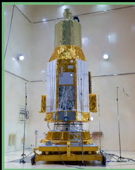
XRISM acoustic test at JAXA's Tsukuba Space Center in December 2022. CREDIT: JAXA
