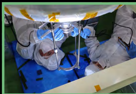
De-integration of the Resolve instrument due to the dewar leak by NASA team, beginning with the removal of delicate filters from the Aperture Assembly at the ISAS/JAXA facility in Japan. Left: Samuel Moseley, right: Steven Kenyon. CREDIT: NASA/JAXA
