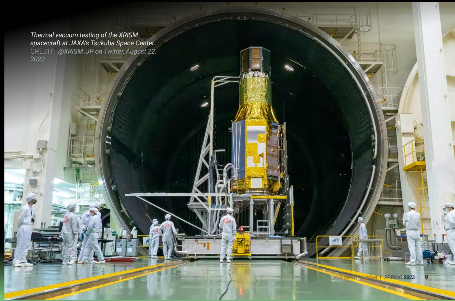
Thermal vacuum testing of the XRISM spacecraft at JAXA's Tsukuba Space Center. CREDIT: @XRISM\_JP on Twitter, August 22, 2022
