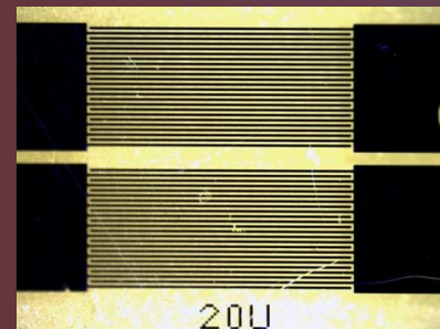
Large Area SiC Diode for LET Detectors
