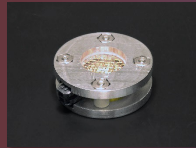
Large Area SiC Diode for LET Detectors
