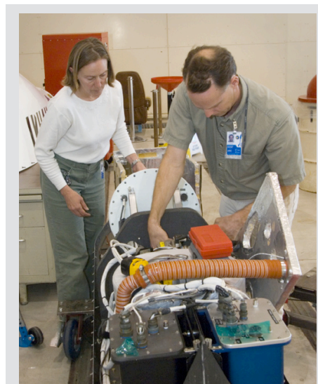
NASA photo NASA Ames engineers Sally Buechel and Ted Hildum prepare to load the Autonomous Modular Scanner into the Ikhana remotely piloted aircraft's payload pod, Oct. 23, 2007 to observe the California wildfires
