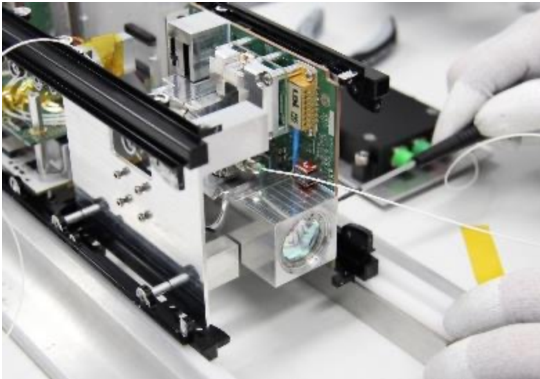
OSIRIS integrated in QUBE satellite
