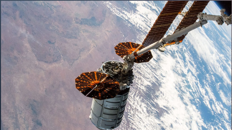
The International Space Station using the Canadarm2 robotic arm to capture a Cygnus spacecraft
