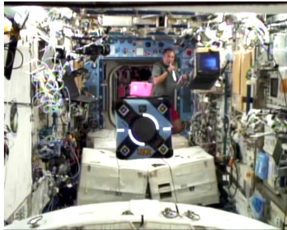
JAXA astronaut Soichi Noguchi pauses to watch Bumble conducting a multi-sensor map survey
