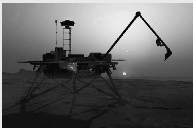
An artist's rendition of the Phoenix lander, by Corby Waste of the Jet Propulsion Laboratory. The Phoenix is scheduled for launch in August 2007 and will land on Mars in May 2008. The lander's robotic arm will dig into the arctic terrain in search of clues about the history of water on Mars and also for evidence of organics.
