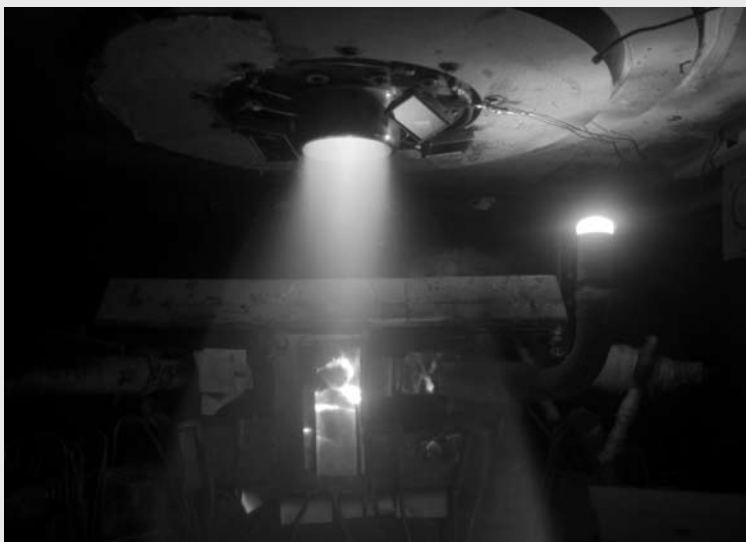
Arc Jet test at the NASA Ames Interaction Heating Facility (IHF) (top view) with thermal protection system (TPS) material coupon glowing after test completion.
