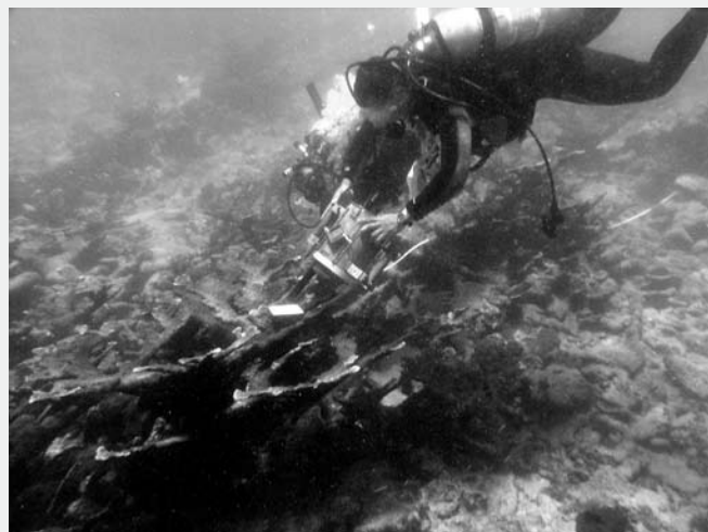
NASA Ames and University of Puerto Rico divers taking a spectral measurement with a handheld spectroradiometer.
