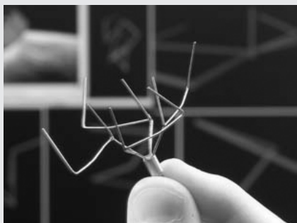
One of the small space computer-designed antennas recently flown aboard the Pegasus XL rocket.
