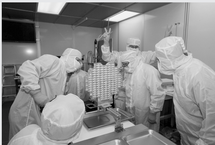
Scientists study the Stardust sample return particles (center) that were captured by Stardust's specialized 'arm' and remained enveloped within the Aerogel substance inside the spacecraft's interior.
