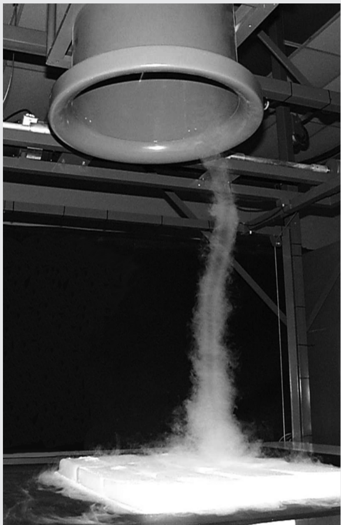
The Arizona State University Vortex Generator, CO 2 visualization experiments.
