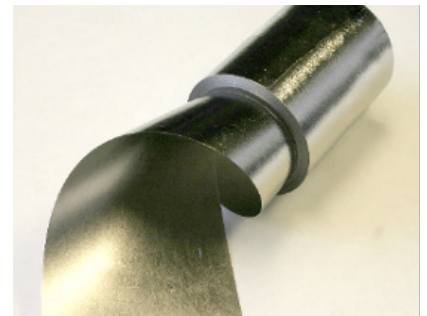
Figure 2 Magnetic Ribbon: New magnetic materials enable vehicle electrification by operating at higher frequencies and temperatures with low power loss.
