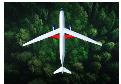
Figure 1: Transonic truss-braced wings can help reduce fuel consumption by up to 10 percent. (NASA)
