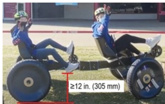
Figure 1. Vehicle Height Requirement
