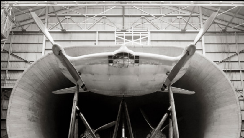
Vought-Sikorsky V-173 STOL fighter concept in FST
