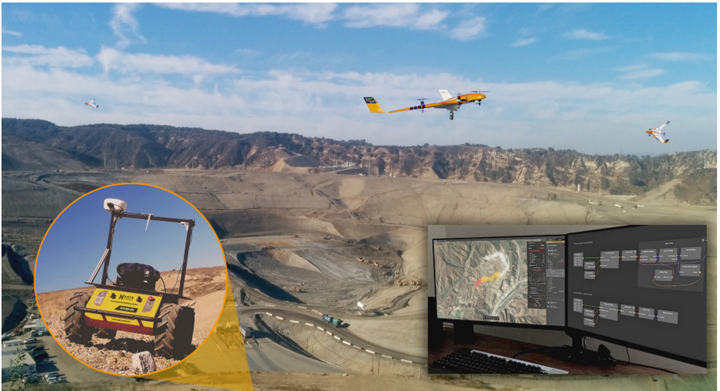
HATS using SWS tools for automated drones and rovers to assess methane emissions at a landfill.
