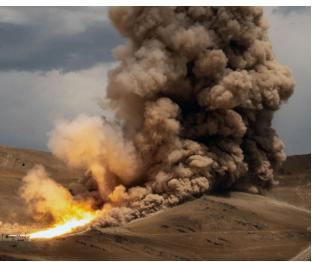
Solid rocket booster motor ground test for future flights of the agency's Space Launch System rocket in Promontory, Utah.
