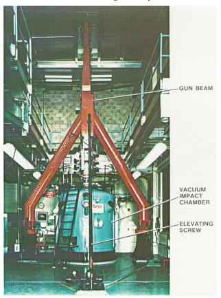
Figure 4.2.2.1. Photograph of the Ames Vertical Gun Range Facility
