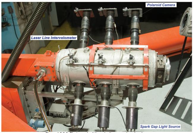
Figure 4.2.2.6. Photograph of the velocity measuring chamber
