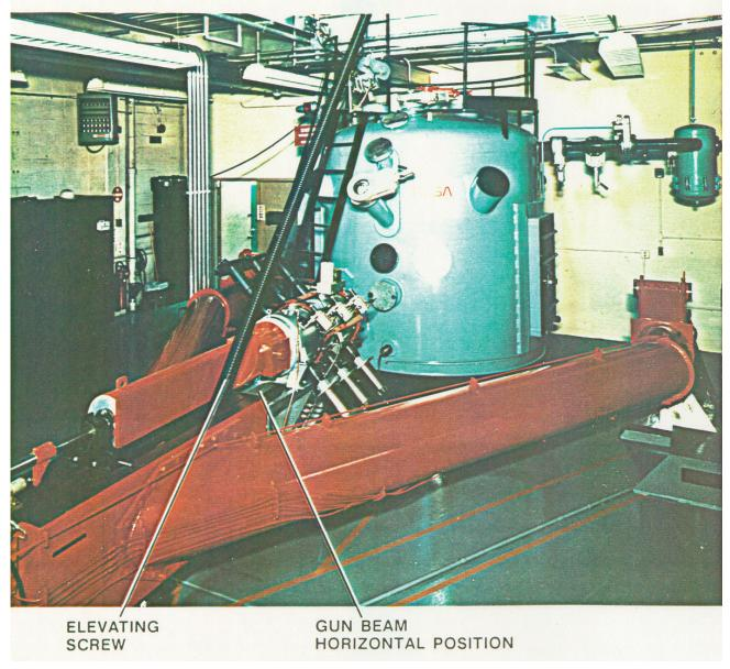
Figure 4.2.2.13. Photograph of gun elevation system, beam in horizontal position
