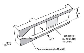
Figure 4.1.2.3. Schematic representation of the TFD nozzle and test section
