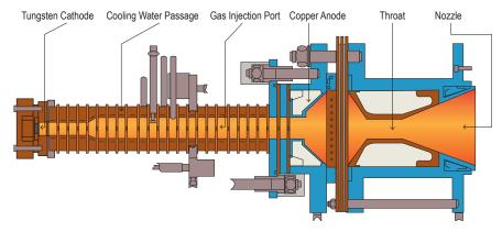
Figure 4.1.1.3. Schematic drawing of the 10 MW dual-bore arc heater
