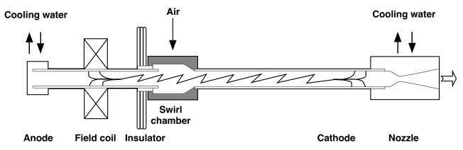
Figure 4.1.1.1. Schematic drawing of the Huels arc heaters used at ARC
