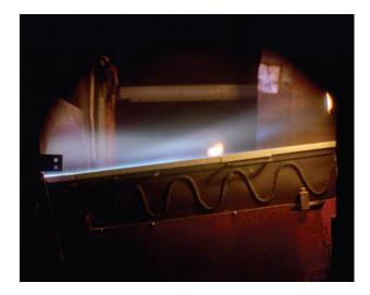
Figure 4.1.0.3. 24×24 in (61×61 cm) panel being tested in the arc jet complex
