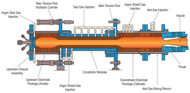
Figure 4.1.1.2. Schematic drawing of the 20 MW and 60 MW segmented arc heaters used at ARC. N.B. Add gas mixing plenum is: not available for PTF; configurable for AHF; standard for IHF
