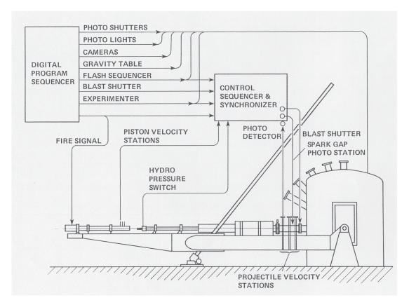
Figure 4.2.2.12. AVGR simplified block diagram
