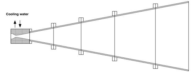
Figure 4.1.2.2. Schematic drawing of a conical nozzle family
