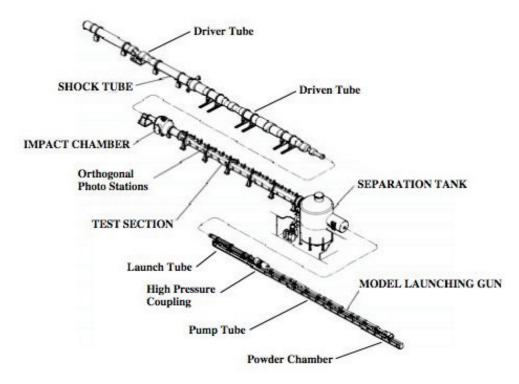
Figure 4.2.1.1. The Hypervelocity Free-Flight Aerodynamic Facility
