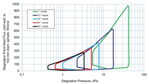
Figure 4.1.3.2. Operating envelope of the AHF with 20-MW segmented arc heater
