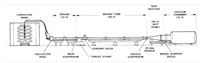
Figure 4.2.3.1. Schematic diagram of the EAST Facility
