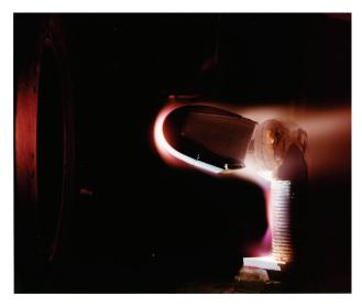
Figure 4.1.0.4. Leading-edge model being tested in the arc jet complex
