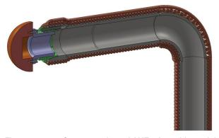
Figure 4.1.4.1. Cut-away view of AHF sting with model
