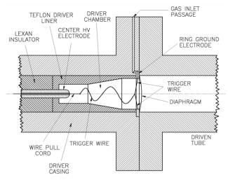
Figure 4.2.3.2. EAST Facility current collector and arc chamber
