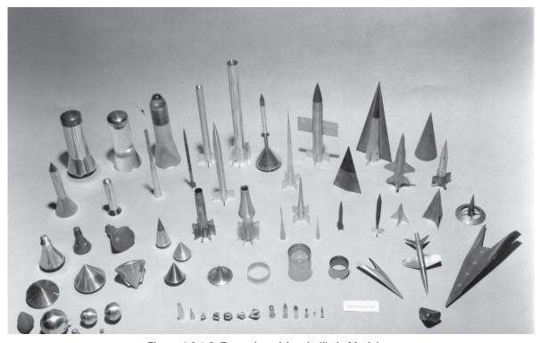
Figure 4.2.1.2. Examples of Aeroballistic Models
