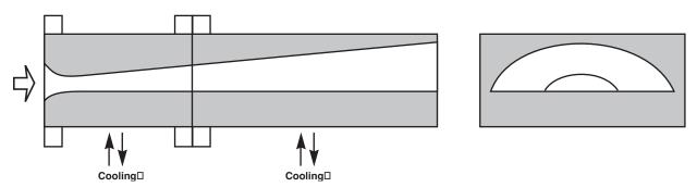
Figure 4.1.2.1. Schematic drawing of the semielliptical nozzles at ARC
