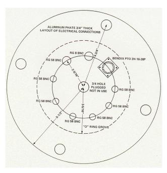
Figure 4.2.2.11. AVGR standard vacuum feed-through plate
