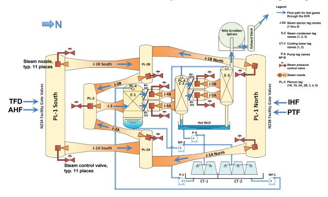
Figure 4.1.6.1. Schematic diagram of the five-stage SVS
