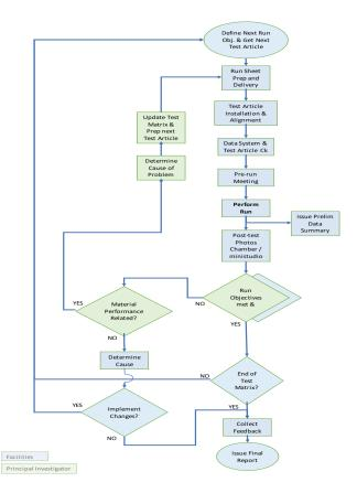
Figure 2.3. Test execution process
