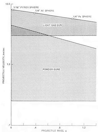
Figure 4.2.2.4. Light gas and powder gun performance
