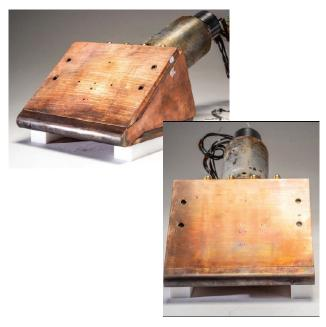
Figure 4.1.5.3. Example of wedge calorimeter probe
