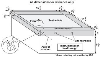
Figure 4.1.4.4. Test fixture assembly for PTF
