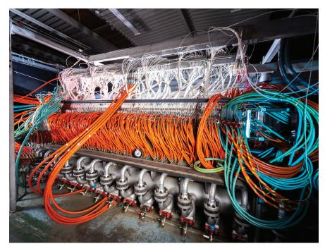
Figure 4.1.3.5. 60 MW segmented arc heater in the IHF
