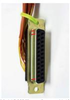
Model D25S Harness Layout with 12 each Type K Thermocouple Wires
