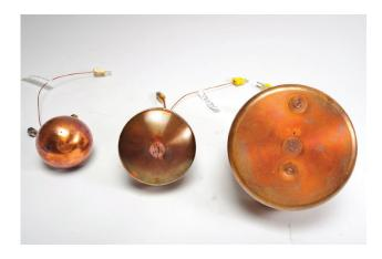
Figure 4.1.5.1. Examples of typical slug-calorimeter probes
