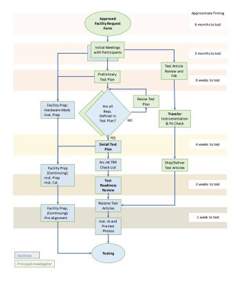
Figure 2.2. Typical test preparation process
