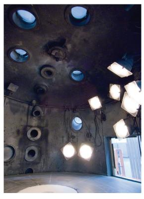
Figure 4.2.2.8. Impact vacuum tank (interior view)
