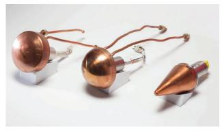
Figure 4.1.5.2. Examples of null-point/coaxial TC calorimeter probes
