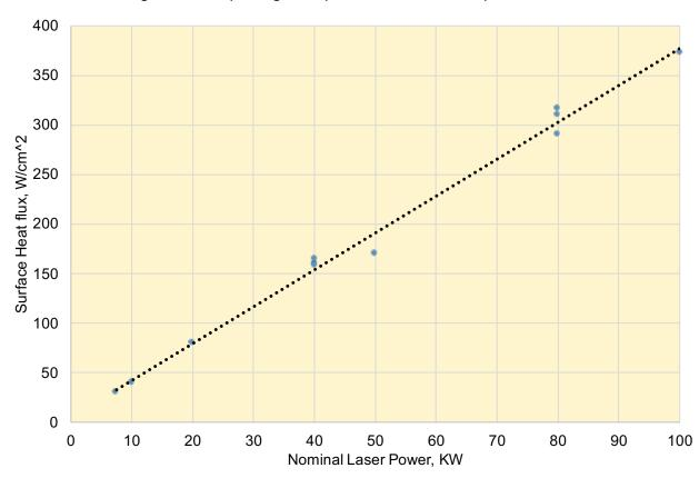
Figure 4.1.3.9. Laser Power vs. Radiant Calorimeter Readings on 6"×6" Target
