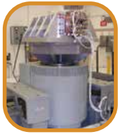
Vibration test of an Environmental Control and Life Support Systems Component
