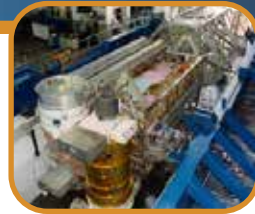
Modal Test of the ISS P3/P4 Truss
