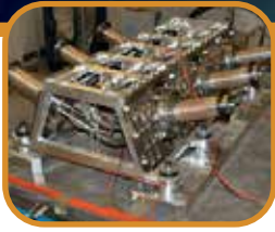
Vibration test of roll control thruster module
