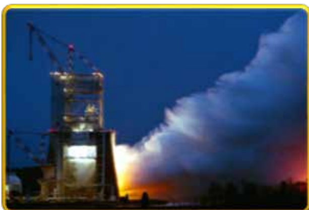
Atlas II AR (RD180 Engine) hot fire at 4670
